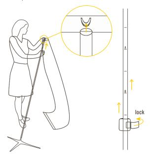
O4 Connect the bottom snap profile to the pole by pushing the pole clip against the pole. Assembly is complete
