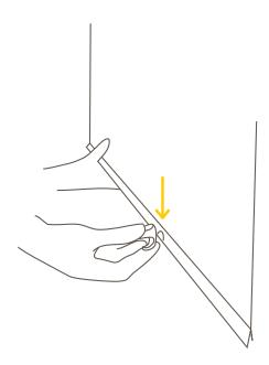
Insert the top connector on the pole to the slot of the top snap profile.
