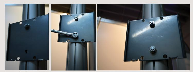
Use the provided Hammerhead Bolts to attach the Monitor Bracket at the desired height. Gently tighten the nuts using the provided wrech. Too much can warp the aluminum post or break the bolt. IMPORTANT: Ensure that a washer is used on both sides of the Monitor Bracket.
