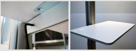
O4 Insert and fasten the Shelf to your desired height using the Hex Key provided. One half turn Right to lock it into place. Do not over turn as this will break the internal lock.
