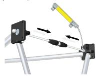
Attach magnetic fastener locks to prevent unintended collapsing of frame.
