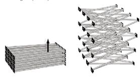
Connect magnetic fasteners to hold the expanded Express display frame in place.
