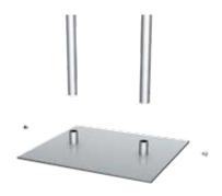
Attach frame onto uprights using Phillips head screws hidden inside frame.
