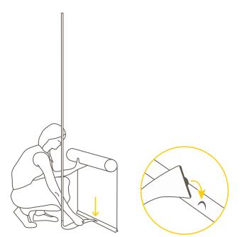
O3 Pull up the graphic panel and bend the pole forward to connect the top of the pole to the slot on the upper graphic profile.
